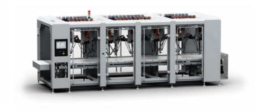
CAMA's in-house developed packagingindustry-specific Delta robot technology enhances our existing range of integrated robotic solutions. This development led to the birth of the Cama Triaflex series – delta robots with carbon fibre arms, suitable for fast and smart product handling. Triaflex can be equipped with an integral highly accurate vision system and can sort and pick loose products on a production line and then position the products into a container or on a conveyor in a pre-set pattern.
