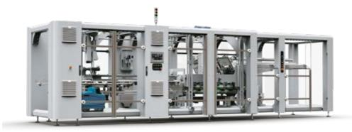
We offer fully digital cardboard sleeving machines for packing bottles, cups, jars, bricks, tins/cans and thermoformed containers in one or two layers from single and/or double lanes. These machines are also suitable for clip-type carton sleeves and bridge sleeves with upper pack hotmelt closing. CAMA's sleeving machines stand out for their technological innovation, high added value, accessibility, ergonomic design, performance, and functionality.
