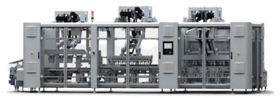
Our 2-axis robotic loading unit, equipped with product-grouping devices, packagephasing conveyors and single or multiple pick-up heads, are designed according to the specifications and features of the customer's product. This unique combination of integrated packaging machines and robotic loading units provides added value by incorporating flexible size changing and high reliability all within a reduced footprint.
